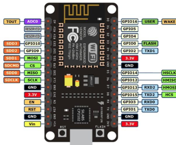
Gambar 2.6 Skema NodeMcu<sup>[5]</sup>
