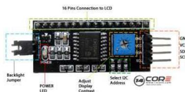
**Gambar 2.13 Susunan Pin Out I2C Serial Interface** <sup>[11]</sup>
