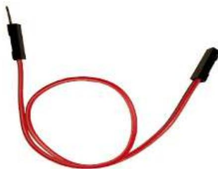
**Gambar 2.8** Kabel Jumper Male To Female<sup>[9]</sup>
