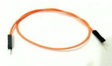
**Gambar 2.7** Kabel Jumper Male To Male<sup>[9]</sup>
