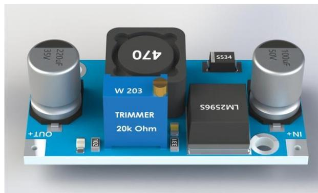
**Gambar 2.4** LM2596 DC to DC Converter Tampak Depan[8].
