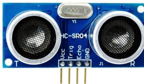
**Gambar 2.9** Sensor Ultrasonik[13].
