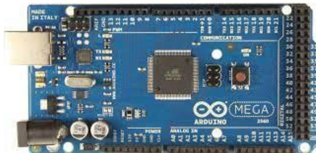
**Gambar 2.9** Arduino mega 2560
