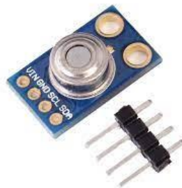
Gambar 2. 4 Sensor Suhu MLX90614
