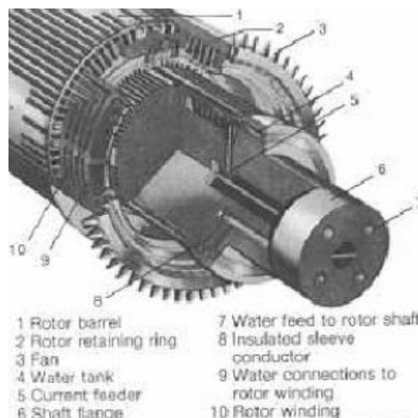
Gambar 2.6 Rotor Kutub Silinder Generator Sinkron 2
