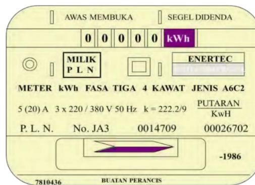
Gambar 2. 12 Contoh Name plate kWh meter
