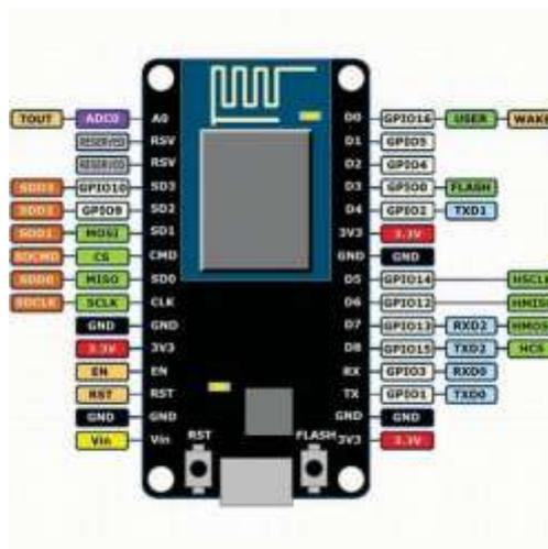
**Gambar 2. 35** Pinout NodeMCU ESP8266 [64]
