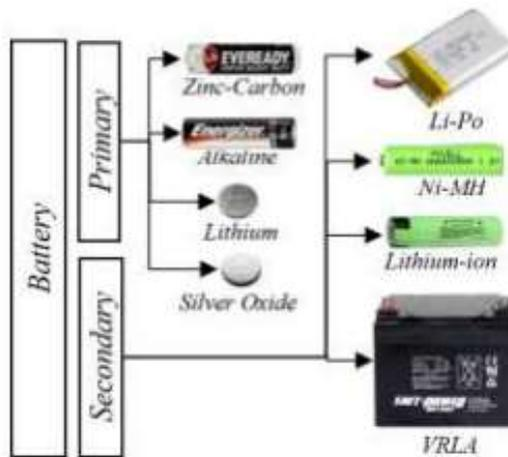
**Gambar 2. 6** Diagram Alur Baterai [3]
