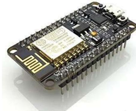
**Gambar 2. 33** NodeMCU ESP8266. [61]
