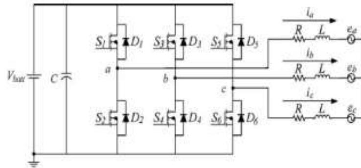
**Gambar 2. 27** Converter circuit with BLDC motor load[55]
