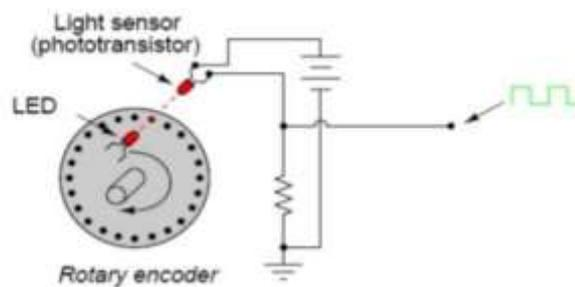
**Gambar 2. 38** Sensor optocoupler
