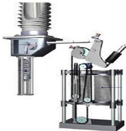
Gambar 2. 7. Sistem Pegas Pilin (helical)
