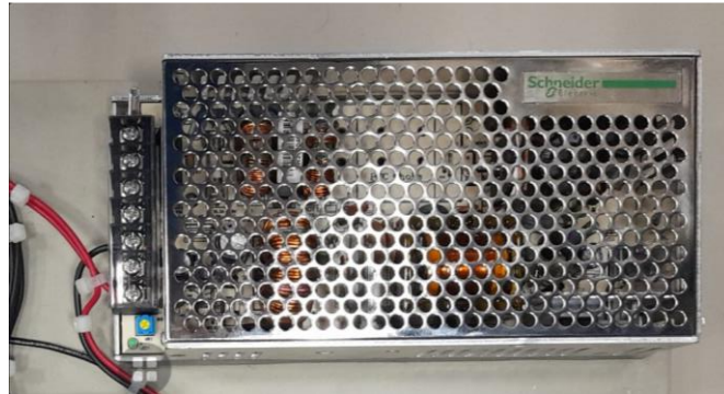
Gambar 2.10 Power Supply Switching
