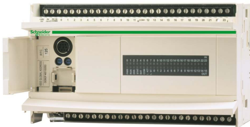
Gambar 2. 1 PLC Compact TWDLCAE40DRF [4]
