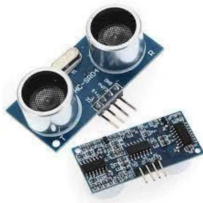
**Gambar 2. 6** *Ultrasonic proximity sensor*
