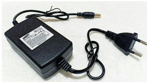
Gambar 2. 9 Adaptor 12V 5A Sumber : https://jadistore.com
