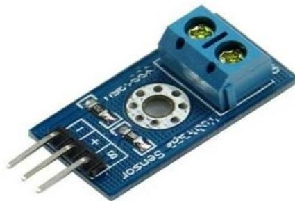
**Gambar 2. 10** Module Sensor Tegangan
