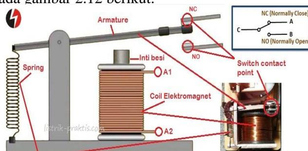
**Gambar 2. 12** Prinsip Kerja Relay
