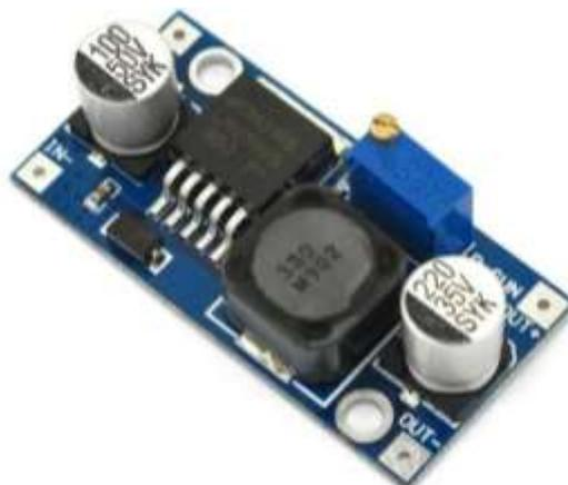
**Gambar 2. 7** Modul *Step Down* DC-DC
