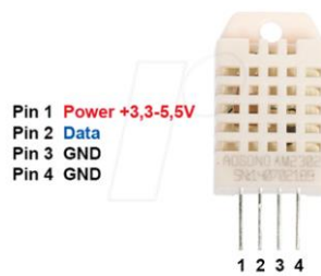
Gambar 2. 5 DHT22 tanpa Resistor Pullup
