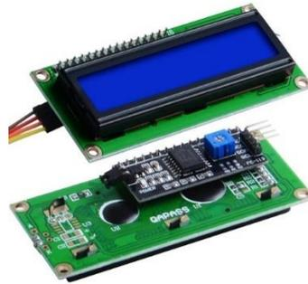
**Gambar 2.19** LCD (Liquid Crystal Display)
