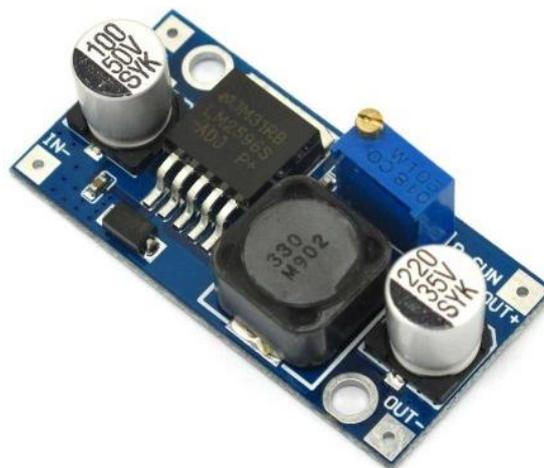
**Gambar 2.18** Modul Step Down LM2596
