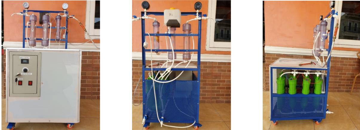
Gambar 1. Rancangan Hydrogen Fuel Generator
