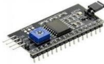
Gambar 2. 6 Modul I2C Backpack LCD
