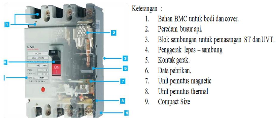
Gambar 2.3 MCCB (*Moulded Case Circuit Breaker*)
