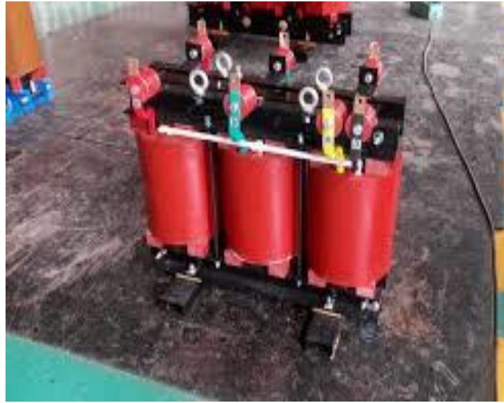
Gambar 2.8 Transformator tipe Kering
