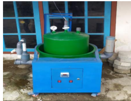
Figure 1. Prototype fixed dome biodigester
