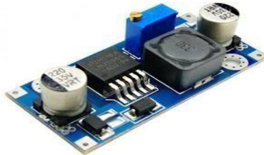
**Gambar 2. 9** Modul Step Down DC LM2596
