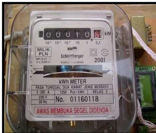
**Gambar 2.6 kWh Meter Analog**
