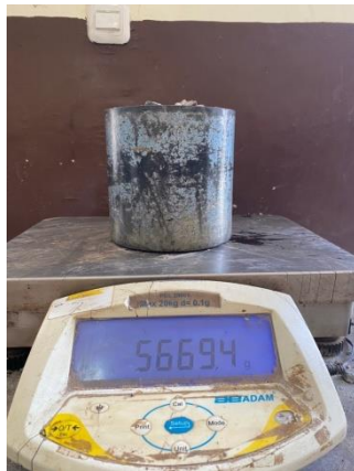
Penimbangan bobot isi gembur agregat 1/2 sample 2
