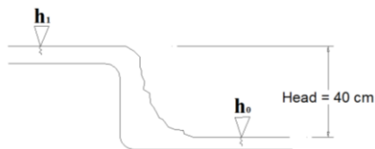
Fig. 2 Sketch of the Head measurement at the research site.
