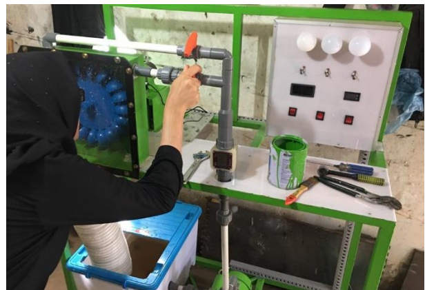
Figure 2. Operation of Prototype of Micro Hydro Power Generation Equipment
