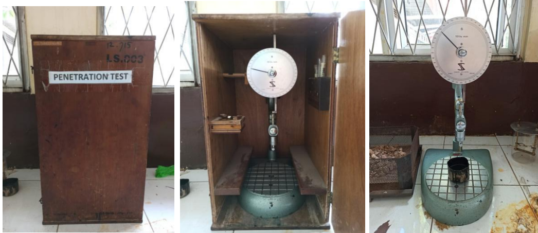
1. Alat Penetrasi Aspal / Penetration Test
