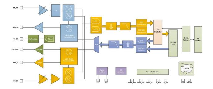
• SX1276/77/78/79 is a half-duplex, low-IF transceiver. Here the received RF signal is first amplified by the LNA. The LNA inputs are single ended to minimize the external BoM and for ease of design. Following the LNA inputs, the conversion to differential is made
