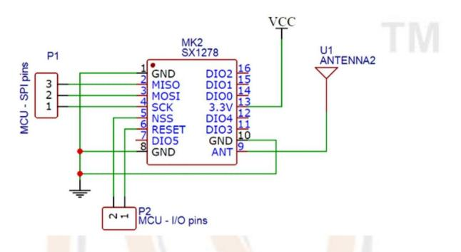
• To communicate with the module some standard libraries are also available for Arduino like LoRa by Sandeep and other platforms. The module comes in a surface mount style package hence care should be taken while soldering. It is also a common practice to solder wires and pins with the module to use it as through hole module.
