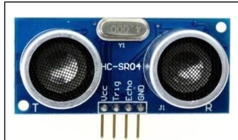
**Gambar 2. 5** Sensor Ultrasonik HC-SR04
