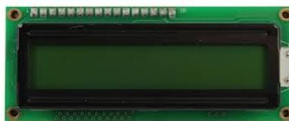
**Gambar 2.12 Liquid Crystal Display(Suyadhi, 2010)**
