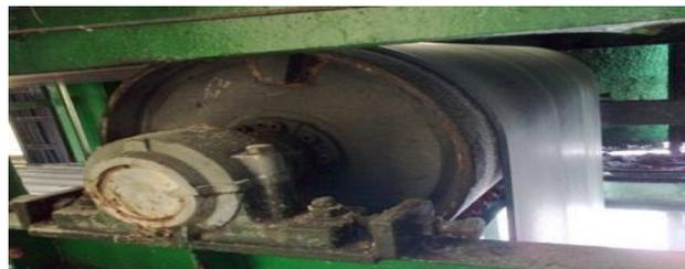
Gambar 2.19 *Bend Pulley*
