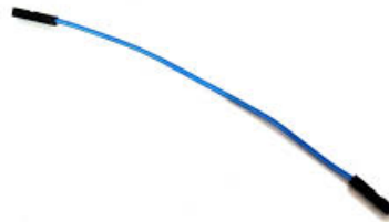
Gambar 2.14 Kabel Jumper Female to Female
