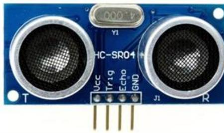
**Gambar 2.19** Sensor Ultrasonik HC-SR04
