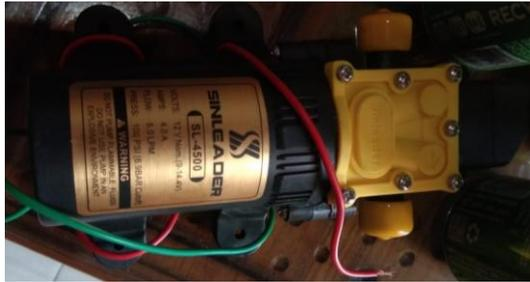
**Gambar 2.30** Pompa Air DC 12 Volt
