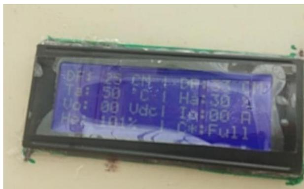
**Gambar 2.27** LCD (Liquid Crystal Display) 20x4
