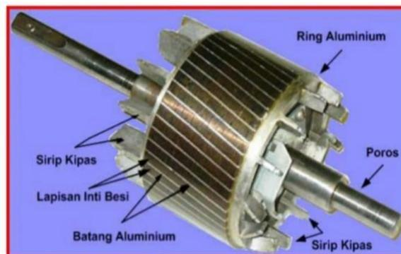
**Gambar 2.7.** Motor Rotor Sangkar
