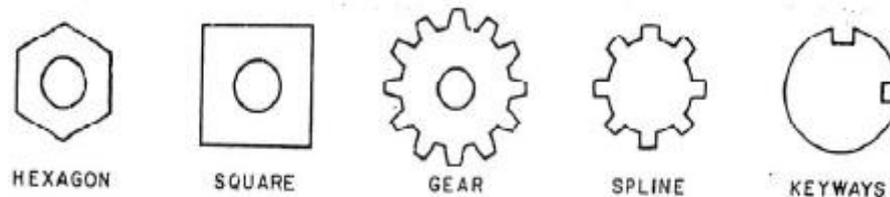
**Gambar 2.16** *Komponen Fixture Indexing* (Hilman, 2019)
