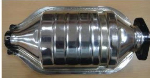
Gambar 2. 2 *Catalytic Converter*
