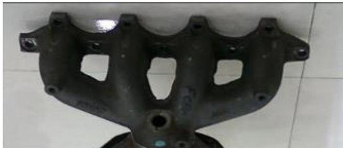
Gambar 2. 1 *Exhaust Manifold*
