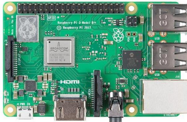
**Gambar 2.6** Raspberry Pi 3 Model B+<sup>[7]</sup>
