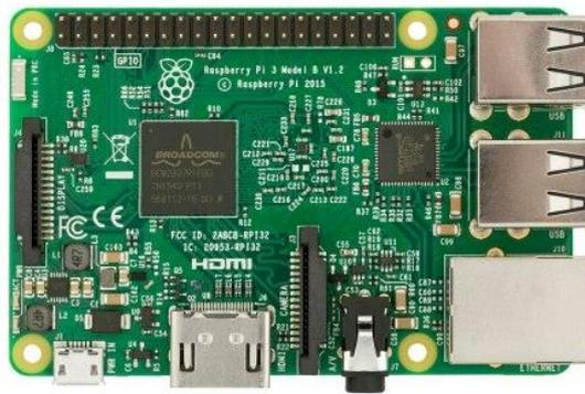
**Gambar 2.5** Raspberry Pi 3 Model B [6]
