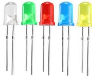
Gambar 2.7 LED ( Light Emitting Diode )
