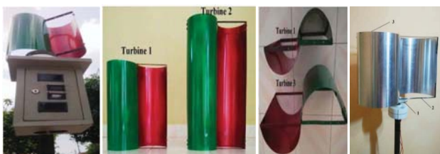
Figure 2. VAWT Control panel with 2 different height and size turbine blades
