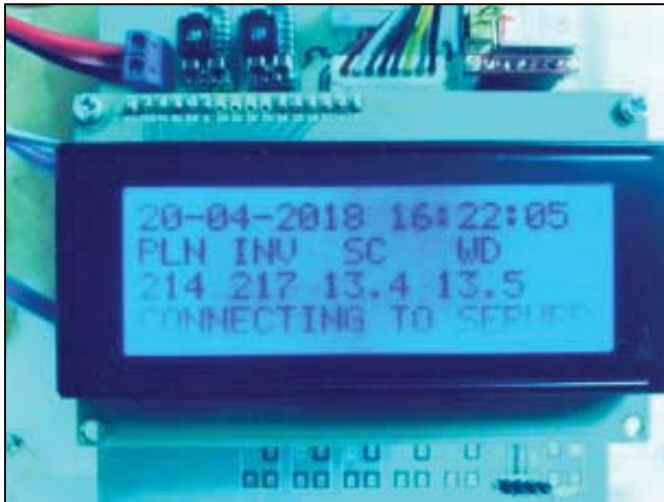
Figure 8. LCD 20 x 4 Sainsmart IIC/I2C/TWi Serial 2004 module shield
