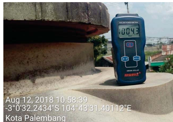
Figure 6. Solar meter for measuring irradiance.
