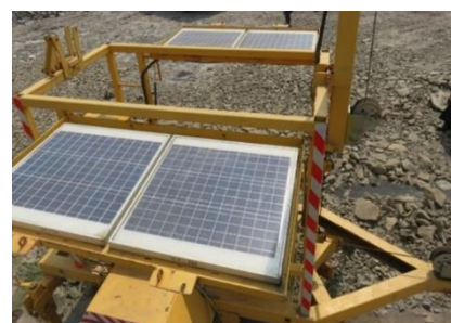
Figure 2. The PV panels to power mobile tower deployed in the open-pit mine.
