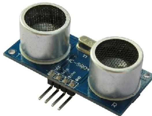
Gambar 2.27 Sensor UltraSonic HC-SR04
