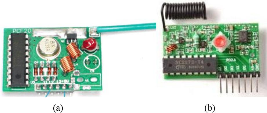
**Gambar 2.4 Modul Radio Frekuensi (a) *Transmitter* (b) *Receiver***
