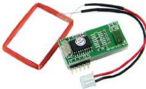
Gambar 2.1 Reader RFID ( Radio Frequency Identification )
