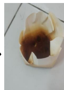
pencucian sampel dgn 50 ml aquadest (5x)
