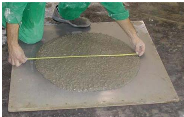
Gambar 2.5 pengujian slump flow
