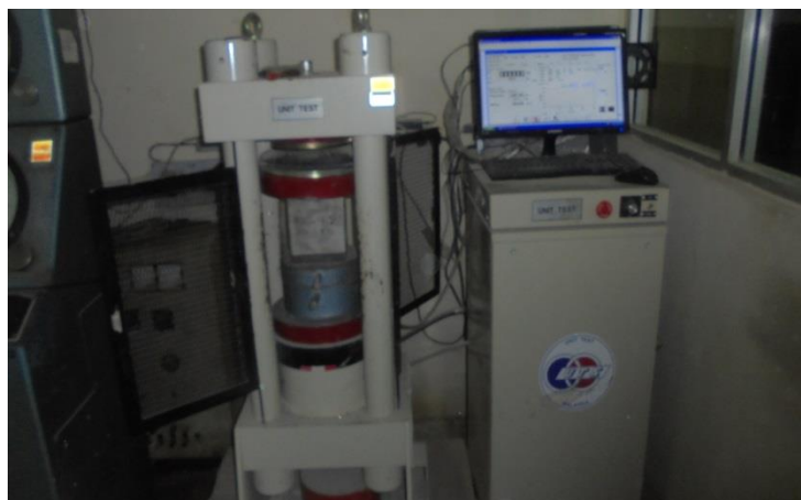
Gambar 2.3 Alat Pengujian Kuat tekan Beton (compression testing machine)
