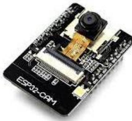
**Gambar 2.7** Esp32-CAM
