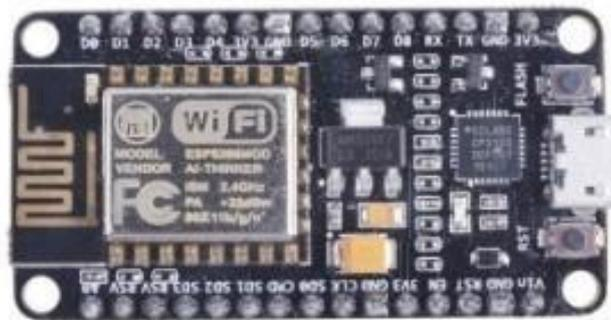
**Gambar 2. 5** NodeMCU ESP8266
