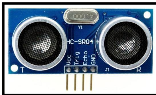
**Gambar 2. 2 Sensor Ultrasonik**
