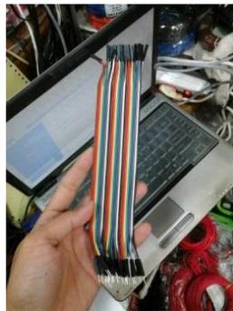
**Gambar 2. 5 Kabel Jumper**
